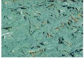
A polysaccharide tackifier increases the surface bond to debris, including plastic and other slick-surface materials, ultimately lowering blowing debris and transing orders
