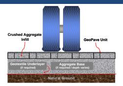
Figure 1 The GeoPave Porous Pavement System
