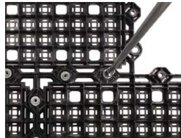
Figure 13: Installing Bolts with Manual Bolt Drive Tool
