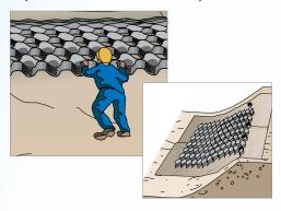
5 Toe in GEOWEB® at the upstream termination.
