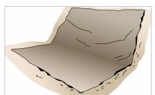
Expand GEOWEB® wall sections with Method A, B or C. Infill sections.
