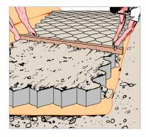
9 Install GEOWEB® layers as specified. Assure minimum 2 inch (50 mm) set back.
