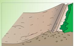
Install geotextile with overlaps (per manufacturer's recommendations if required)
