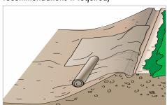
3 Secure sections with ATRA® anchors at the top of the slope. See options A, B.
