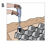
4 Expand sections down the slope.
