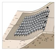
6 Connect GEOWEB® sections with ATRA® keys. Connect side to side (A) and end to end (B).
