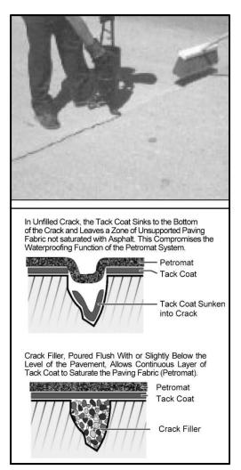
Fill cracks flush with or slightly below the existing pavement surface. If cracks are overfilled, such that the filler mounds up above the surface of the pavement, a noticeable bump in the pavement can result. This can lead to shoving of the overlay or bleeding of excess asphalt.
