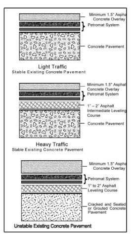
This leveling course should be 1" to 2" thick. The asphalt concrete mix should leave a relatively smooth surface after compaction. Do not use an open, coarse mix, because this will allow the tack coat to seep down into the pores, leaving inadequate tack coat to saturate the paving fabric.
