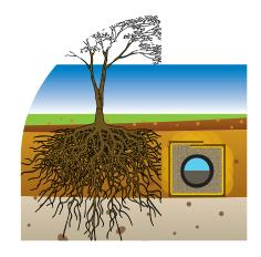
Tree roots seek out air and moisture in the soil, causing expensive damage to underground infrastructure. BIOBARRIER'S unique geotextile design lends flexibility to surround infrastructure, extending the life of your investment
