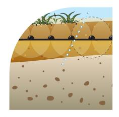
Installed horizontally below three inches of stone/wood mulch, the BIOBARRIER weed control system blocks weeds using two layers of defense: chemical and physical.
