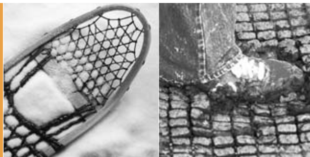
Figure 1: The Snowshoe Effect – Tensar BX Geogrids distribute heavy loads over soft soils just like a snowshoe supports the weight of a man over soft snow.
