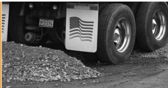
Figure 12: Geogrid can be trafficked directly by rubber-tired equipment.
