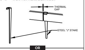
3c USE A STEEL HAIRPIN LEAVING A GAP FOR THERMAL EXPANSION
