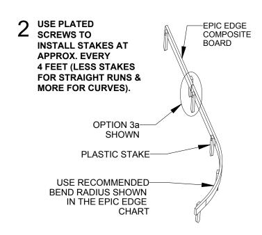
3a USE TWO STANDARD STAKES MOUNTED ON OPPOSING SIDES LEAVING A GAP FOR THERMAL EXPANSION. USE PLATED SCREWS TO JOIN BOARD TO STAKE.
