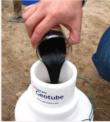
RDT test setup.
