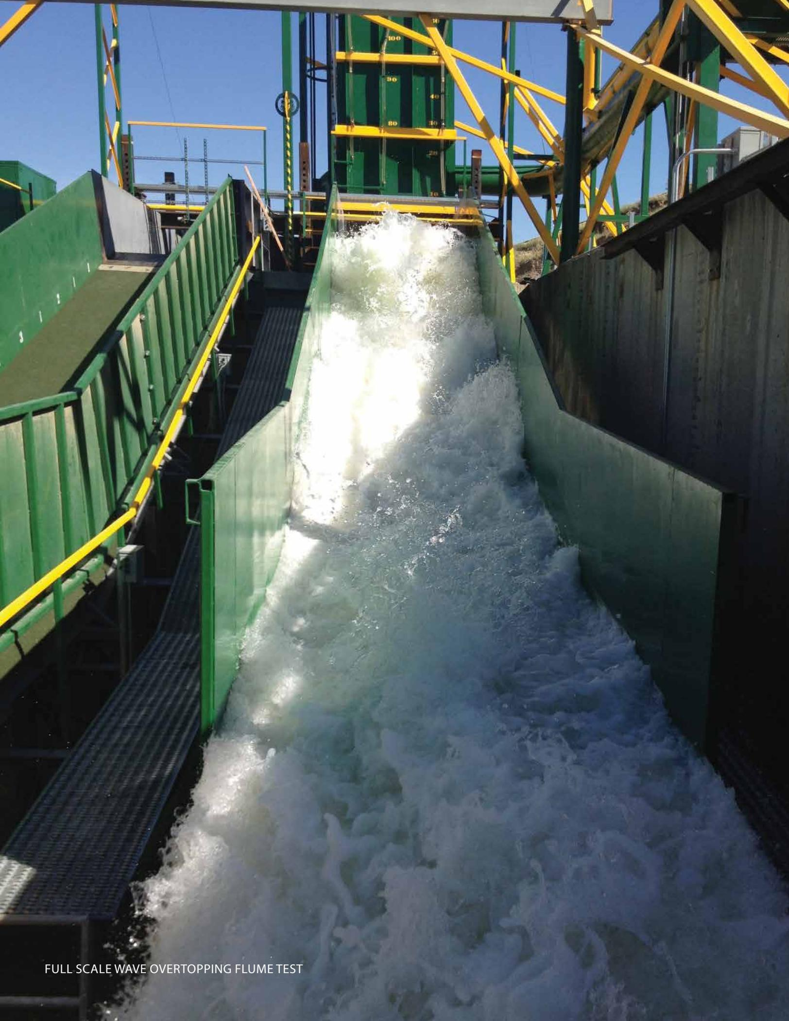
FULL SCALE WAVE OVERTOPPING FLUME TEST
