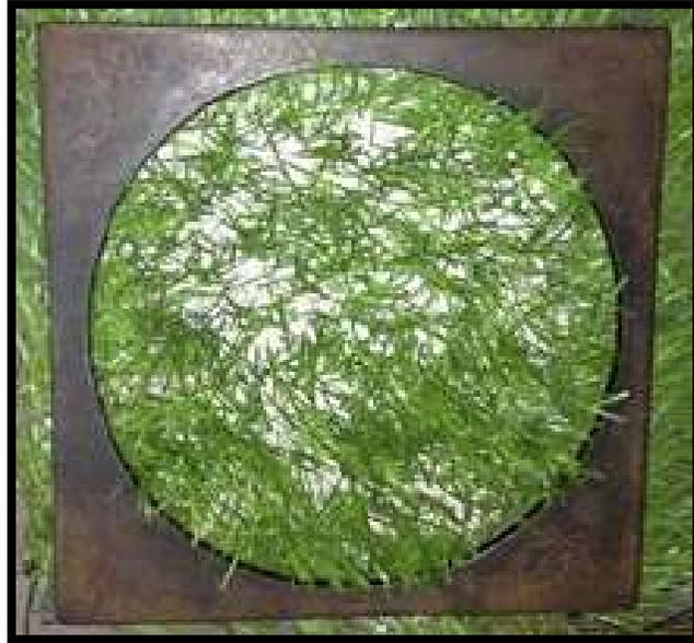
**Figure 1. HydroTurf® Sample Prepared for Flammability Testing**
