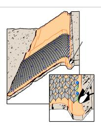
Figure 4 Placement of Geoweb® Section
