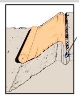
Figure 2 Geotextile Placement
