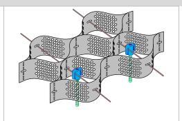
Figure 13 Internal Anchors
