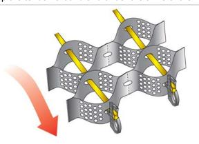
Figure 11 Termination of Integral Tendons
