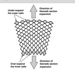
Figure 8 Tapered Expansion of Section
