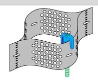
Figure 3 ATRA® Stake Anchor Placement
