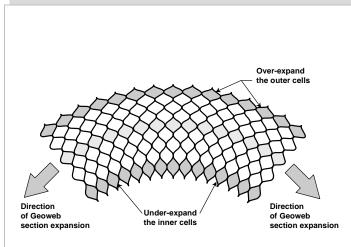
Figure 7 Curved Expansion of Section
