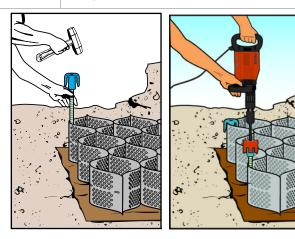
Figure 5 ATRA® Anchor Installation Methods
