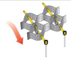
Figure 12 End Anchorage of Tendons
