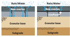
Cracks allow surface water to infiltrate the pavement structure, compromising the strength of the granular base and subgrade.
