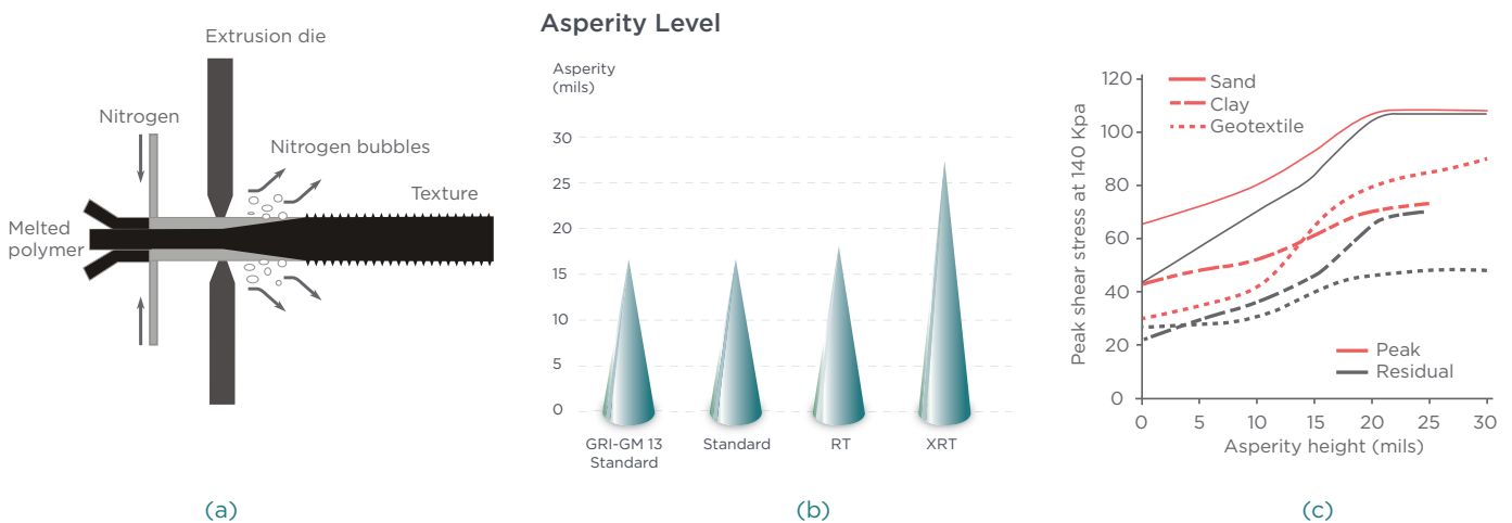
Figure 8: (a) Geomembrane texturing with the blown film co-extrusion method (After Blond and Elie, 2006) (b) Asperity height variations (c) Asperity height vs peak interface shear stress
