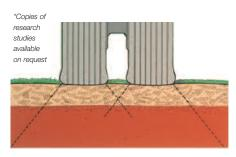
Netlon Advanced Turf distributes the load more efficiently to reduce rutting.
